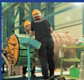
Single multiple layer helical windings are preferably used for low / medium voltage with moderate no. of turns and higher current.
