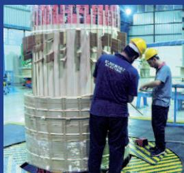
Interleaved disc windings or contra shield disc windings are used for high voltage (132 kv. And above) coils. These types of windings provide better performance during all impulse conditions by making uniform voltage distribution throughout the complete height of the winding.
