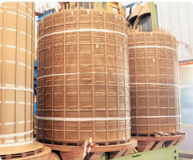
The vertical type machines are used for high-voltage, low-current conditions with a small number of conductors and implements a complex winding method.
