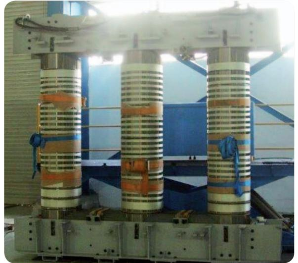
The tapped winding helps to adjust the transformation ratio to network conditions safely, simply, and gradually – whether off load, via tapping switches, or under load, by means of on-load tap-changers.
