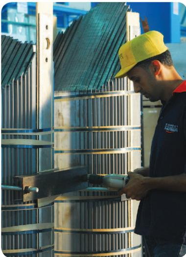
The step lapped joints of the core laminations reduce the additional losses arising in the corner portions
