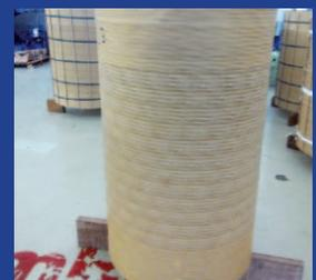
Disc type of windings is suitable for windings with higher no. of turns and with low current. i.e. especially high voltage windings.
