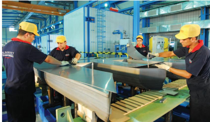
The suitable construction of the frame structure, the preset surface pressure of the lamination, the proper flux density and the gluing of laminations edges after clamping ensure a moderate level of magnetic noise and prevent increase of no-load losses after impulse voltage tests.
